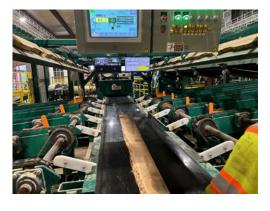
while offering features like a top-mounted sawbox for better maintenance access. The edger operates at feed rates of up to 20 pieces per minute, helping to maximize board yield. **More on OptiFit Edger**.
